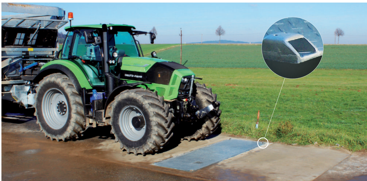
Axle recognition through light barriers.
