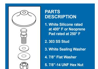
inside the lower cone of the bin along areas where material tends to stick or bridge. By combining both aeration and vibration, the Airbrator can resolve some of the more difficult material flow applications that aeration alone cannot.
